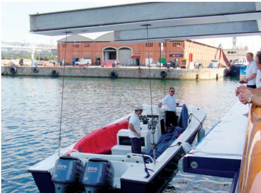
Tender Boat Crane SWL 2.5t + 2x(1.75t) Outreach 5455mm Class LR
