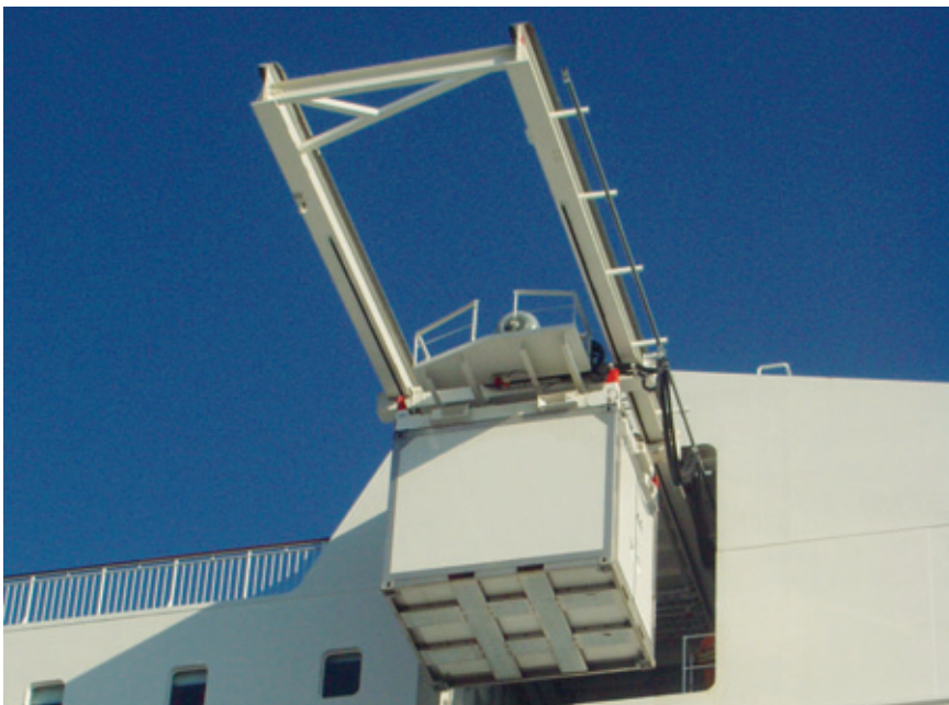
Container Crane SWL 7.5t Class: BV Outreach: 8m
