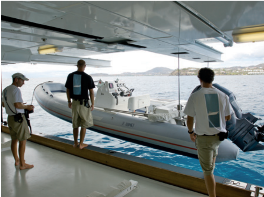
Tender Boat Crane Outreach 3050mm Class LR SWL aftb 2t / fbdy 1t
